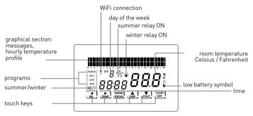
N.B.: to switch on the display, press in the middle; if no other keys are pressed, the display switches off after 2 seconds; if other keys are pressed, the display will switch off after remaining idle when the time set in the parameter LIGHT ON expires [see Chap. 6 CONFIG. PG03].
