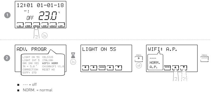
■ A.P. = access point (allows you to connect the smartphone)
