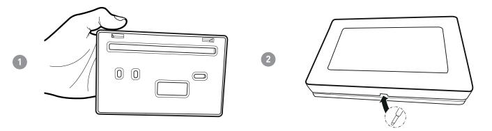
Remove the insulating protection by unscrewing the specific waterproof screw.
