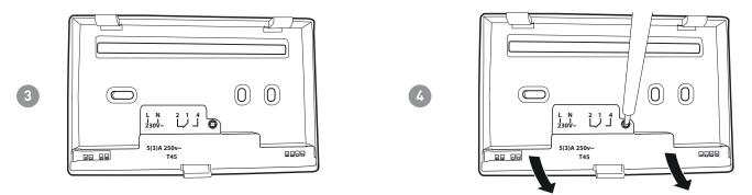
Make the electrical connections (refer to the "Electrical connections" paragraph) and secure the panel to the wall with the supplied screws.
