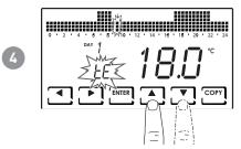
Pressing  $\blacktriangle$  or  $\bigtriangledown$  allows you to select the profile depending on the time. **SETTABLE PROFILES:**
