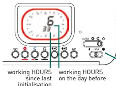
With C57CT the user may verify how many hours the heating system has worked (relay closed - ON) the day before and since the last IntelliTherm initialisation (since last reset or battery fitting).
