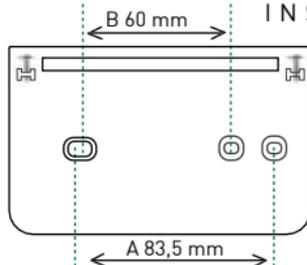
To separate the body from the base for the fitting, remove the batteries cover and loosen from top the two screws, turning the body downwards.
